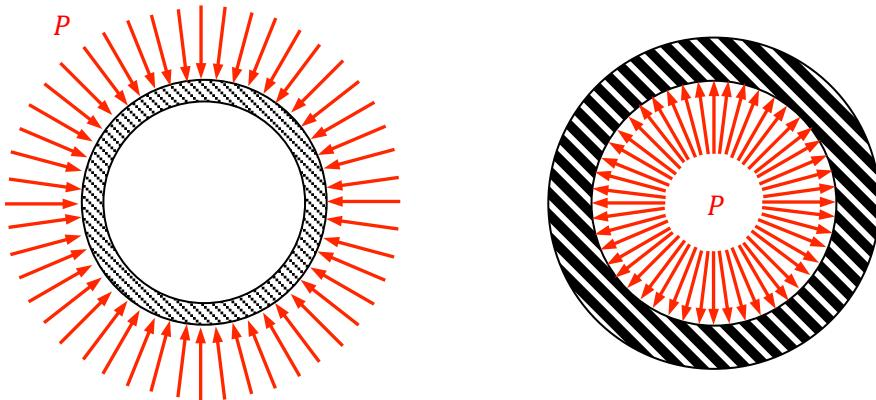
$$u_r^{(1)}(b_1) = -\frac{(1-\nu)(b_1^2/a_1^2)b_1 + (1+\nu)b_1}{E(b_1^2/a_1^2 - 1)}P = -(9,71 \times 10^{-13})P$$
