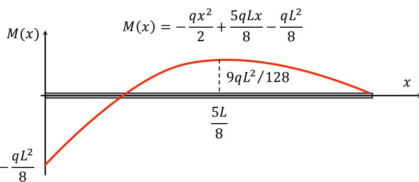
$$\max\{|\sigma_{xx}(x, y)|\} = \frac{h}{2} \frac{\max\{|M(x)|\}}{bh^3/12} = \frac{6}{bh^2} \frac{qL^2}{8} = \frac{3}{4} \frac{qL^2}{bh^2} < S_Y \Rightarrow q < \frac{4}{3} \left( \frac{S_Y b h^2}{L^2} \right)$$
