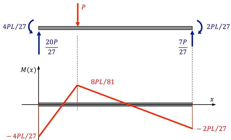
$$\max\{|\sigma_{xx}(x, y)|\} = \frac{h}{2} \frac{\max\{|M(x)|\}}{bh^3/12} = \frac{6}{bh^2} \left( \frac{4P_Y L}{27} \right) < S_Y \Rightarrow P_Y = \frac{27}{4L} \left( \frac{bh^2 S_Y}{6} \right) = \frac{27 M_Y}{4 L}$$
