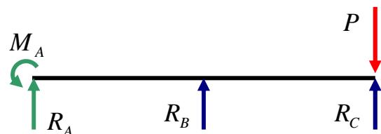
$$R_A = P - (R_B + R_C) = \frac{256 - 48(kL^3/3EI)}{7(kL^3/3EI)^2 + 288(kL^3/3EI) + 256} P$$
