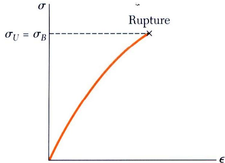
**Fig. 2.11** Stress-strain diagram for a typical brittle material.
