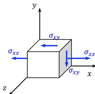
$$[\sigma] = \begin{bmatrix} \sigma_{xx} & \sigma_{xy} & \sigma_{xz} \\ \sigma_{yx} & \sigma_{yy} & \sigma_{yz} \\ \sigma_{zx} & \sigma_{zy} & \sigma_{zz} \end{bmatrix} = \begin{bmatrix} \frac{32PL}{\pi D^3} & -\frac{4PL}{\pi D^3} & 0 \\ 0 & 0 & 0 \\ 0 & 0 & 0 \end{bmatrix}$$
