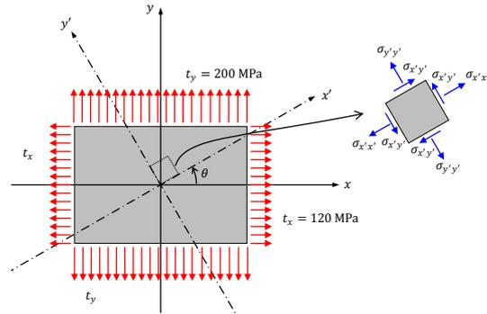
$$\sigma_{x'x'} = \sigma(30^\circ) = \frac{\sigma_{xx} + \sigma_{yy}}{2} + \frac{\sigma_{xx} - \sigma_{yy}}{2} \cos 60^\circ + \sigma_{xy} \sin 60^\circ = 140 \text{ MPa}$$
